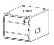
SUB110V and SUB110VW is a high power compact subwoofer made with 1 ferrite magnet 10" drivers that can deliver a peak SPL up to 122dB.
